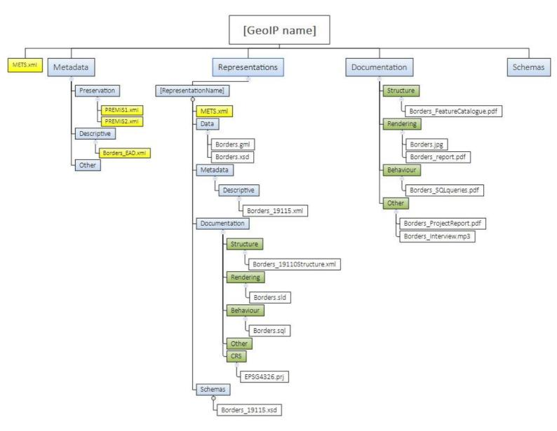
Figure 4. Example Information Package folder structure
