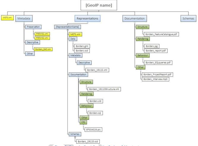
Figure 8 - Example of an Information Package folder structure
